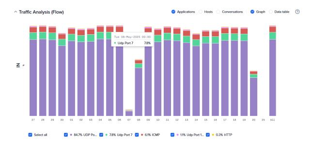
For fast identification of the causes of high utilisation, Flow in Highlight presents 10 minute granularity for the past hour, then smoothing data into hourly, daily and weekly summaries.
